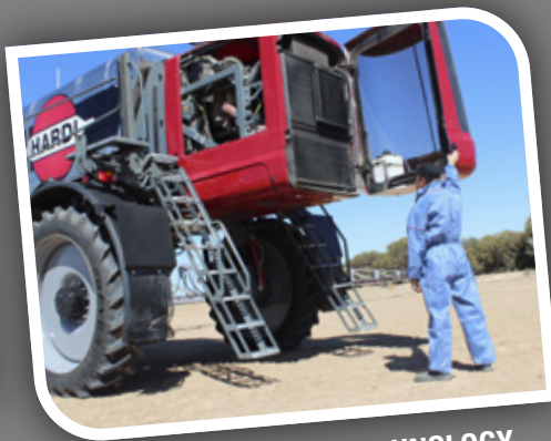
ADVANCED ENGINE TECHNOLOGY RUBICON is powered by Cummins® 8.9l, Tier 3 Engine, 330 or 370 HP Cummins engine
