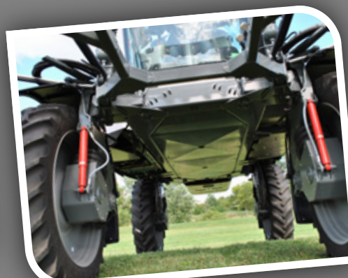
HYDRAULIC TRACK ADJUST The RUBICON axle track width can be adjusted, on-the-run, from 3.0 m to 4.0 m The integrated air-ride suspension provides superior ride and performance.
